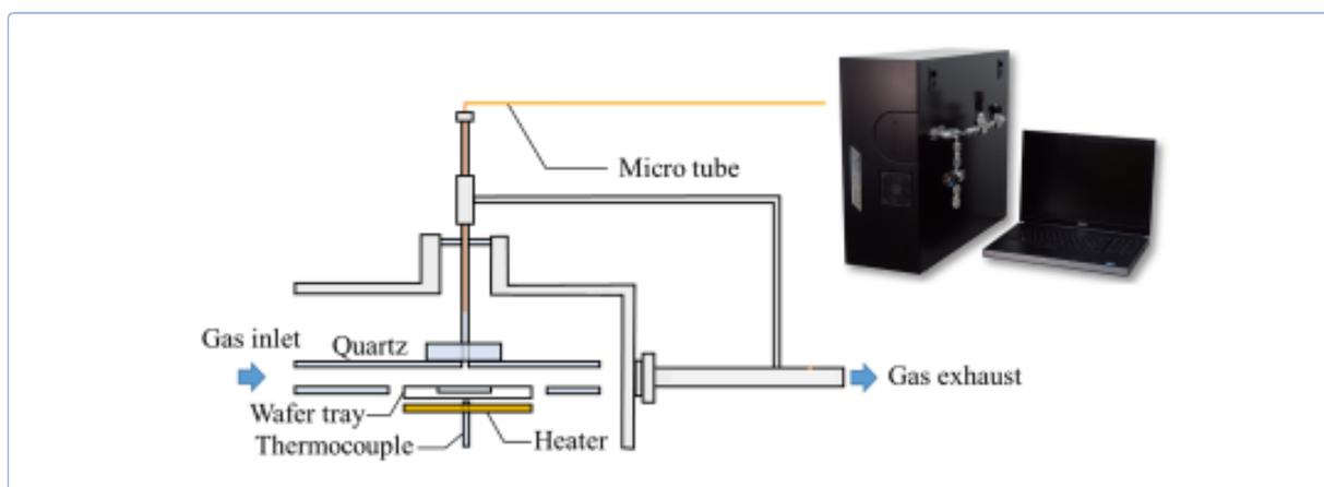
Fig. 1 Experimental setup of MOVPE reactor coupled to the infiTOF-Pro.
