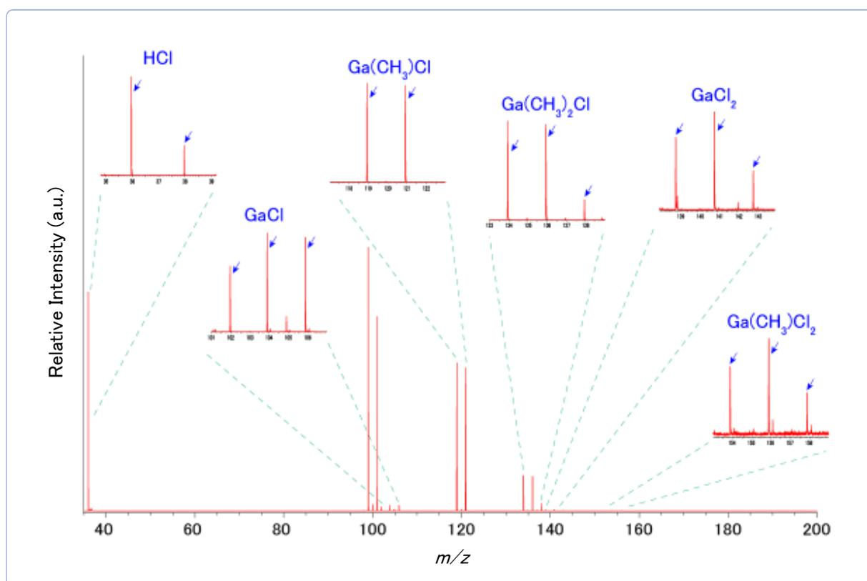
Fig. 3 Mass spectrum of reaction products of TMG and HCl.
