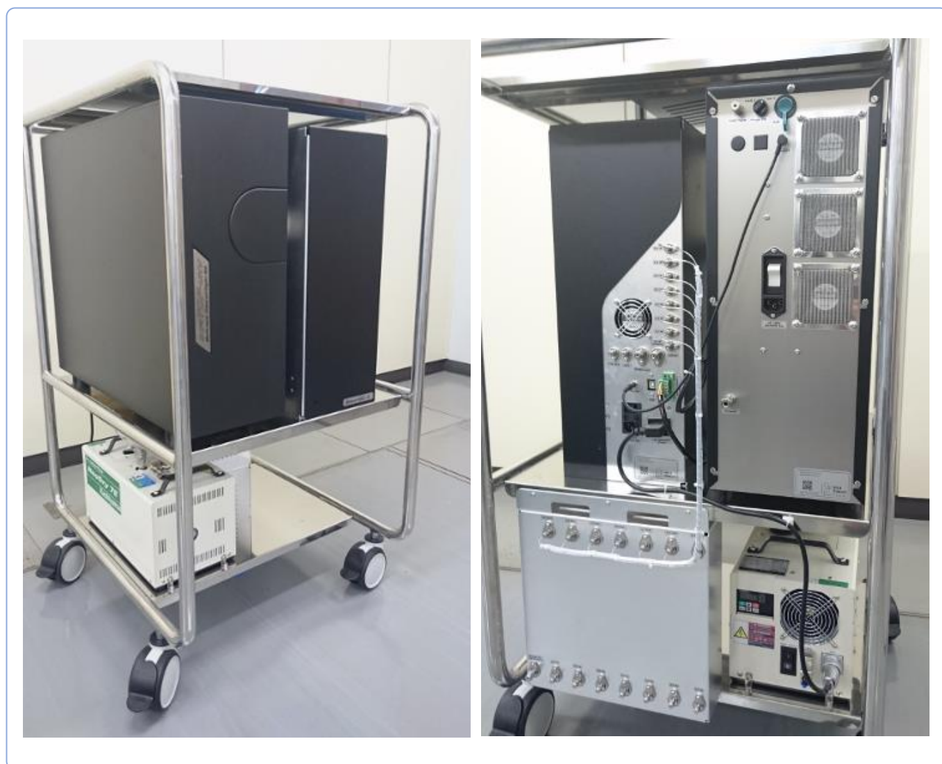
Fig. 1 The smartGC-infiTOF system with seven sampling ports
